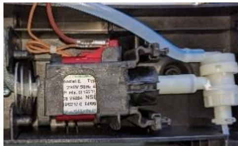
Figure 4.8, Pump inside EC685M
